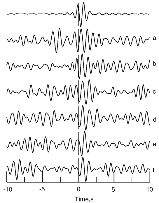
Fig. 7. Examples of waveforms stacked with respect to the theoretical travel times of grid points whose semblance values are relatively high (labeled a–f in Fig. 5). Lines in the each indicate the theoretical travel time for each grid. The uppermost trace is waveform stacked with respect to one grid point on the CMB, where PcP energy is coming. In other traces relative large amplitude wavelets are seen just after the theoretical travel time.
